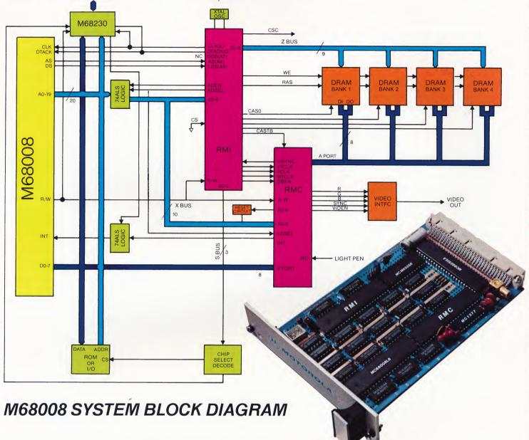
**RMS System** The MPU-based System is quite straightforward and uses primarily VLSI devices. The major elements are the desired MPU, the RMS chip set, one to four banks of dynamic RAM, some "glue" and a video interface part. Additional RAM and I/O parts can be easily attached. The RMS itself consists of two parts: the Raster Memory Interface (RMI) and the Raster Memory Controller (RMC).
